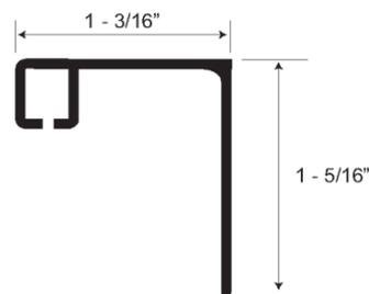
**Section Size:** 1 3/16" x 1 5/16" x .062" wall thickness; extruded of 6063-T5 aluminum alloy; finish is 204-R1 satin anodized. Tab aperture is milled into top of track.
