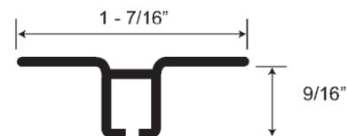
**Section Size:** 1 7/16" x 1 9/16" x .062" wall thickness; extruded of 6063-T5 aluminum alloy; finish is 204-R1 satin anodized. Tracks can be custom fabricated to size and shape with 12" radii bends up to 20' total length.
